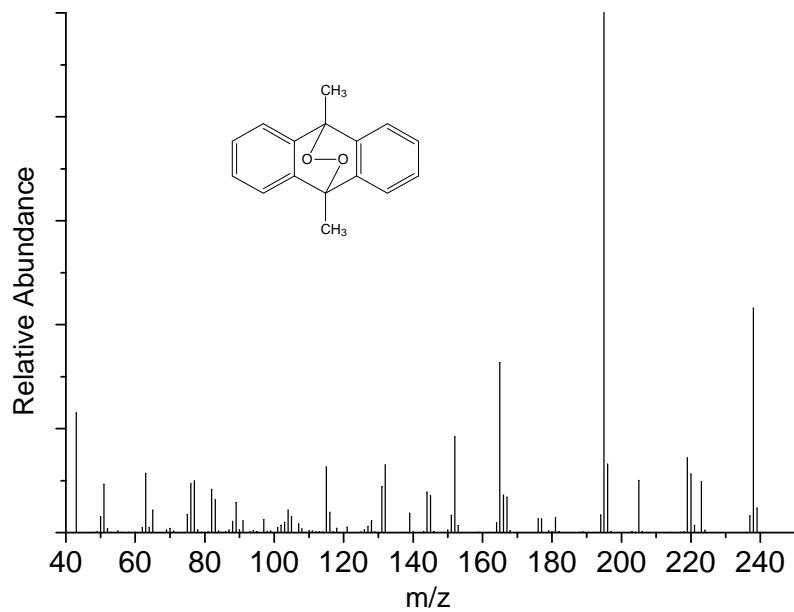
**Figure S2:** MS spectra of DMA endoperoxide.
