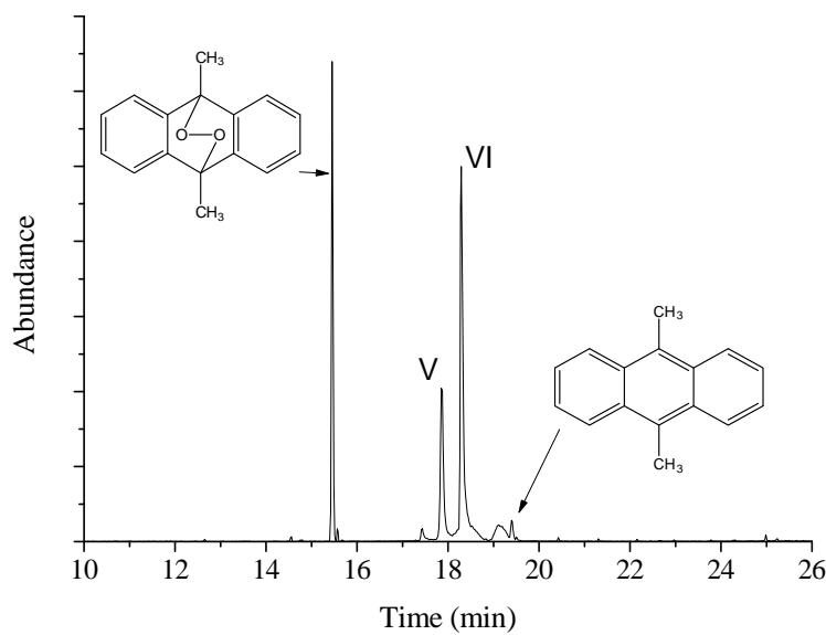
**Figure S1:** GC-MS chromatogram of DMA photooxygenation reaction using SiO<sub>2</sub>-MB nanocomposite.
