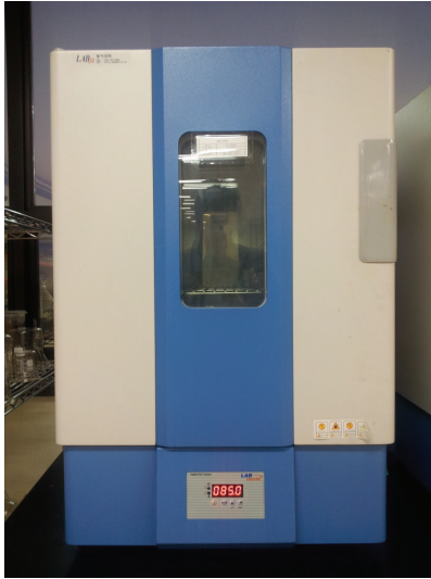
FIGURE 6: Heat test chamber.
