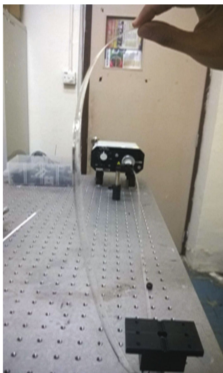
FIGURE 20: Flexibility test of RGOF for bending and twisting mechanism.
