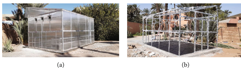
FIGURE 1: Photograph of modified greenhouse dryer structure (a) without and (b) with polycarbonate sheet.
