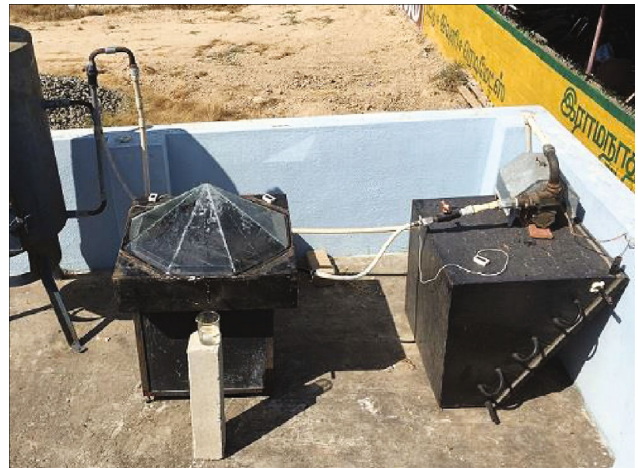
FIGURE 2: Photograph of experimental setup of the octagonal-pyramid solar still.
