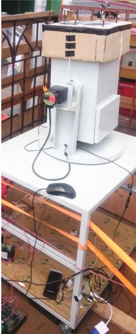
FIGURE 18: Experiment setup of prototype mobile sun-tracking system on a small truck to measure pointing error under moving condition.
