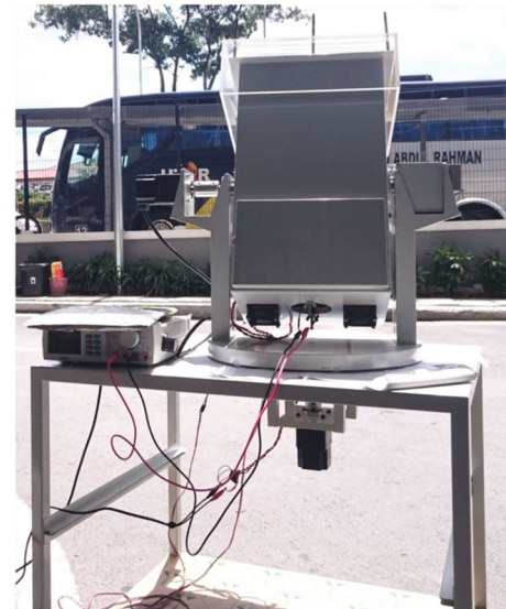
FIGURE 14: Experiment setup to study the pointing error of prototype mobile sun-tracking system under stationary condition.
