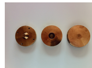
SCHEME 1: Molds used for specimen production of two different forms.
