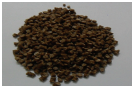
FIGURE 1: Pellets of BBF/PP composites.
