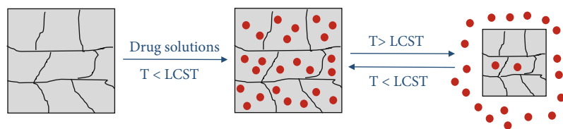
FIGURE 4: Extrusion mode of drug delivery from temperature-sensitive hydrogels.
