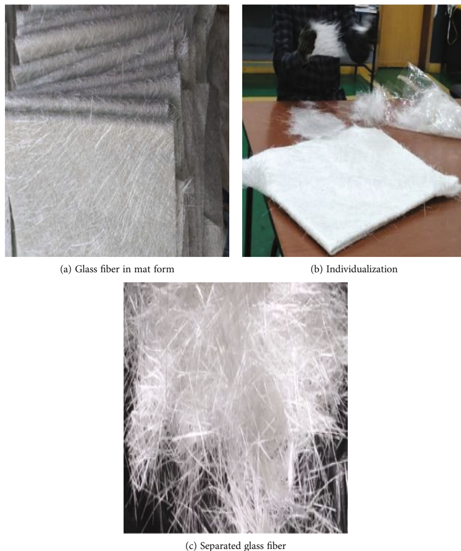
FIGURE 3: Glass fiber individualization process.
