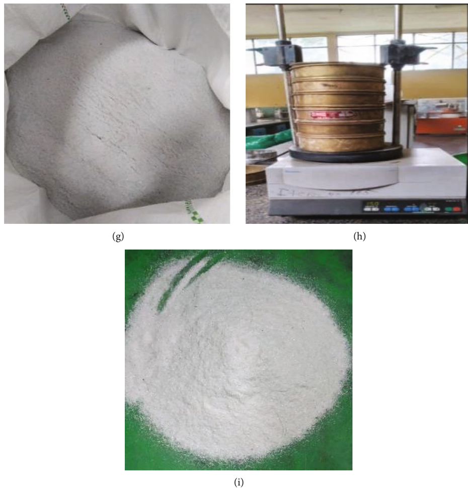
FIGURE 2: Grinding of waste glasses: (a) waste glass collecting, (b) washing, (c) drying, (d) jaw crusher, (e) glass particles after jaw crusher, (f) disk miller, (g) glass particles after disk miller, (h) sieve analyzer, and (i) 0.75-1.0 mm sieve size glass particles.
