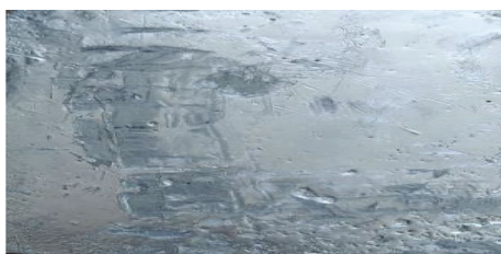
FIGURE 4: Glass fiber-reinforced PET matrix with window glass filler composites.
