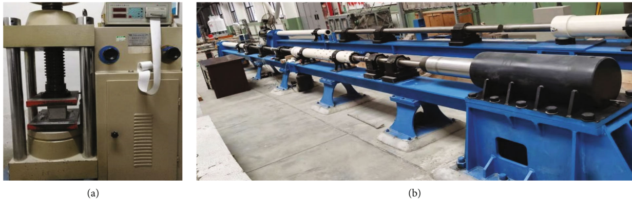
FIGURE 2: Equipment for quasi-static and impact compression tests: (a) servo press tester; (b) split Hopkinson pressure bar.
