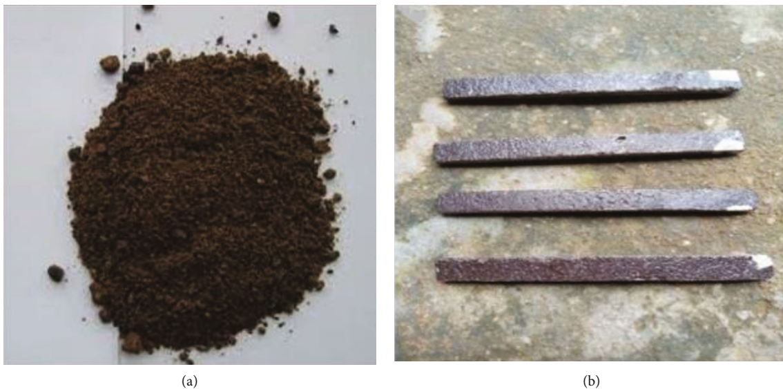
FIGURE 1: Processes to obtain the mold. (a) Powder state of palm kernel shell after grinding, and (b) plastic polyester after the mold from the powder state of palm kernel shell.
