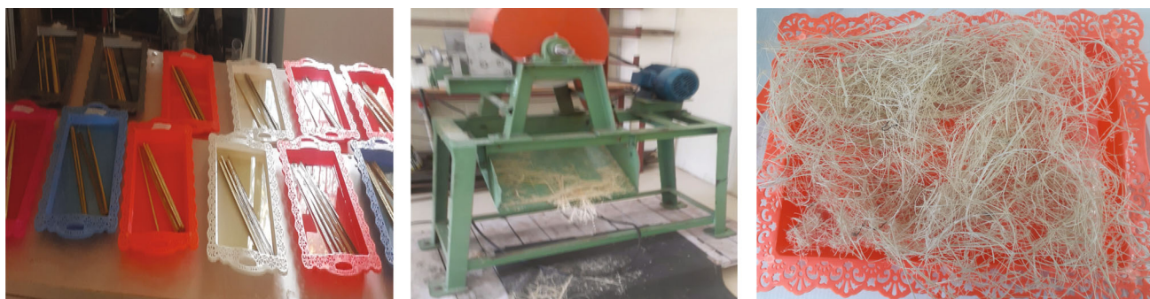
FIGURE 5: Untreated and treated highland bamboo fiber extraction process.
