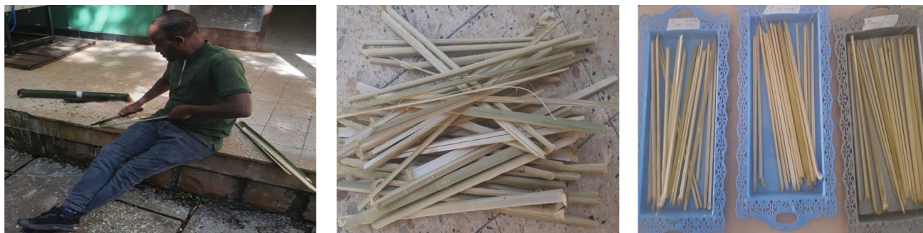
FIGURE 4: Highland bamboo plants were chopped with a slicer.
