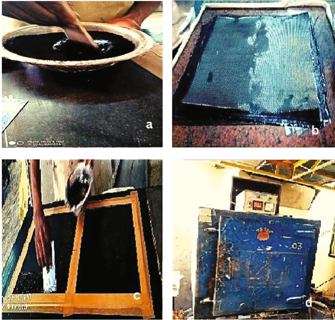
FIGURE 1: (a) Mixing rubber with resin. (b) Spreading carbon fiber over the mixed resin. (c) Alternate layers of mixed resin and carbon fiber. (d) Vacuum bag moulding process.
