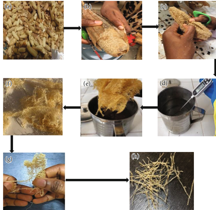
FIGURE 1: (a) Supply. (b) Peeling. (c) Separating the seeds from the sponge. (d) Measuring the water temperature with the thermocouple. (e) Treatment in NaOH solution. (f) Treated Luffa sponge extraction. (g) Manual extraction. (h) Extracted Luffa cylindrica fibre.
