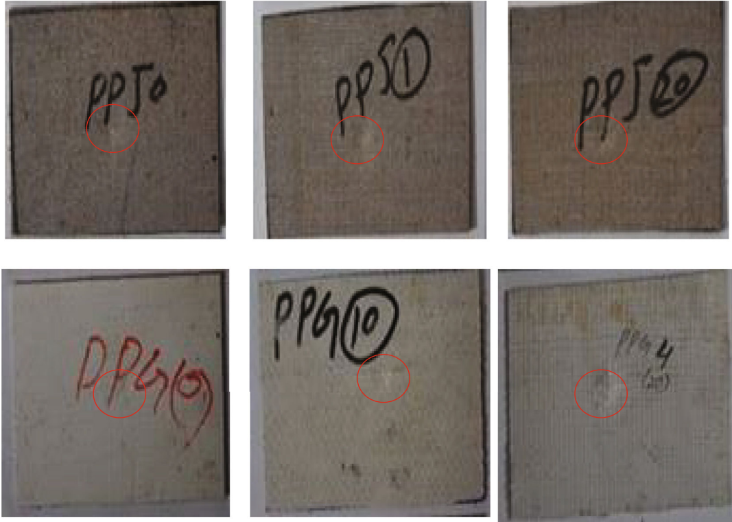
FIGURE 8: Drop weight impact-tested specimen, showing indentation.
