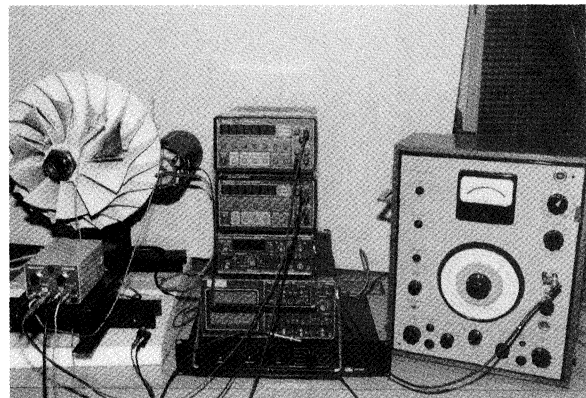
FIGURE 5 Small test stand for investigating the vibration behavior of radial impellers at rest. Excitation by means of a shaker.
