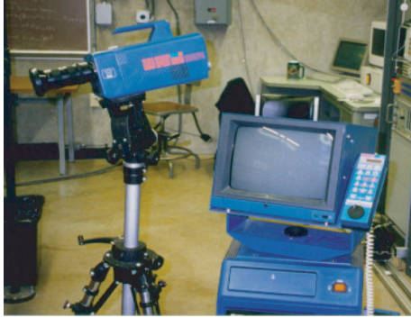
FIGURE 4: View of the high-speed video camera system.
