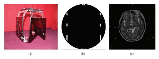
FIGURE 2: (a) A head frame with contrast agent of copper sulphate solution filled in the N shape frames. (b) A CT slice with the frame on. (c) An MR slice at the same head position (same z direction) as that in the CT.
