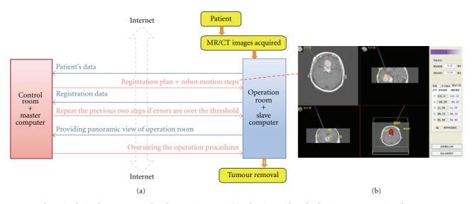
FIGURE 6: Telemanipulation between control and operation rooms (a). Planning path and robotic movements given from master room to the operation room (b).
