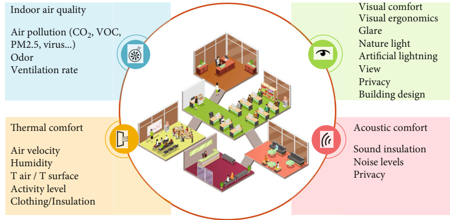
FIGURE 1: Overview of indoor environmental quality.
