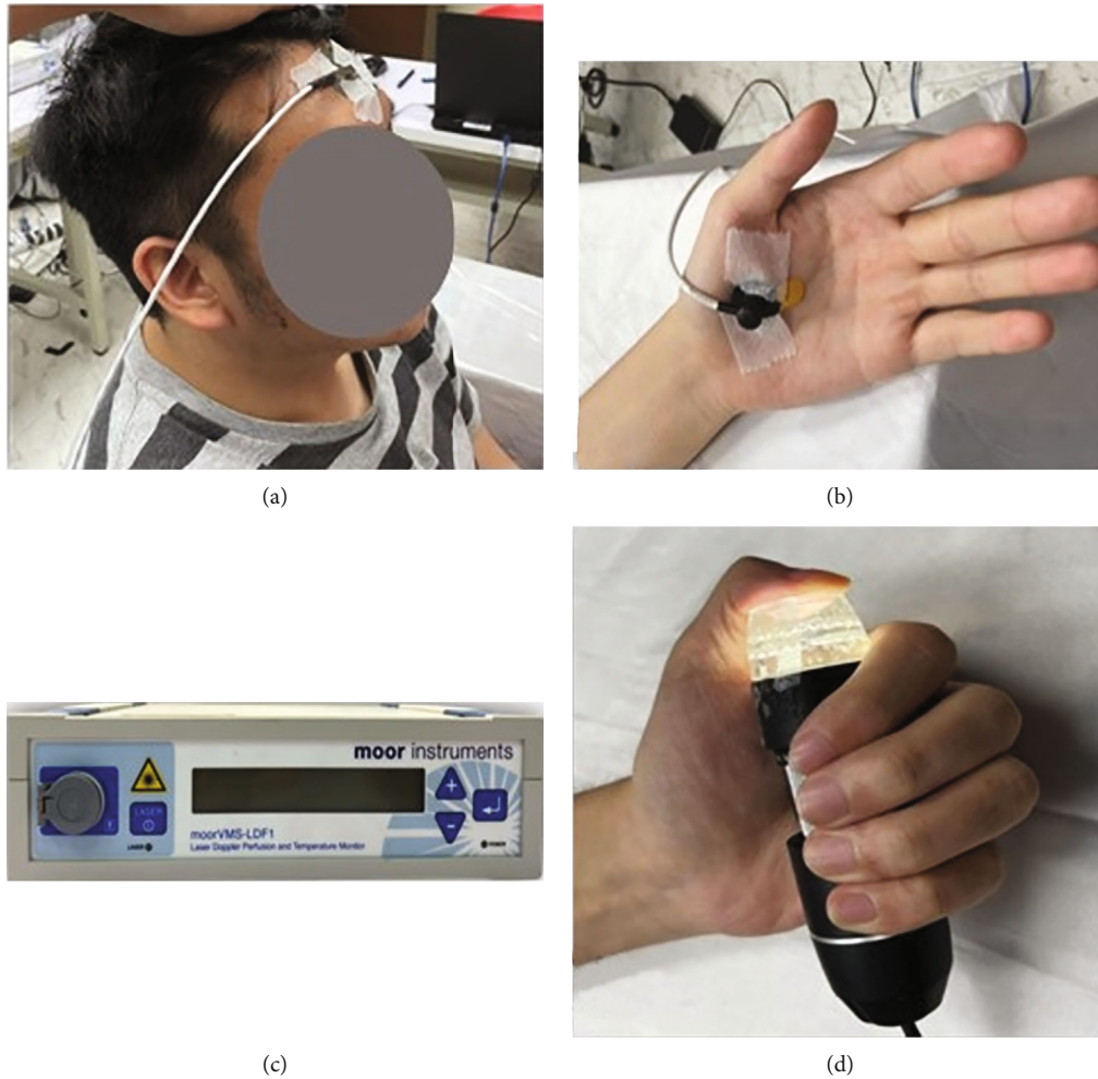
FIGURE 6: Measuring instruments for physiological parameters: (a) skin temperature, (b) SBF, (c) laser Doppler flowmeter, and (d) digital USB microscope for sweat.
