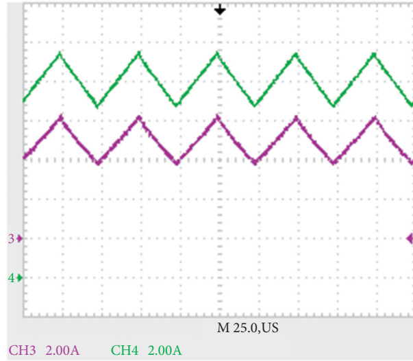
FIGURE 18: Plot of steady-state inductor current I_{L1} (channel-4) and I_{L2} (channel-3) during step-up operation.
