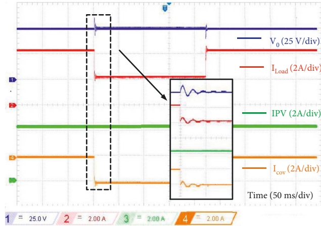
FIGURE 14: Hardware results when the load current is varied from 4.17 A to 2.08 A and vice versa (buck mode).
