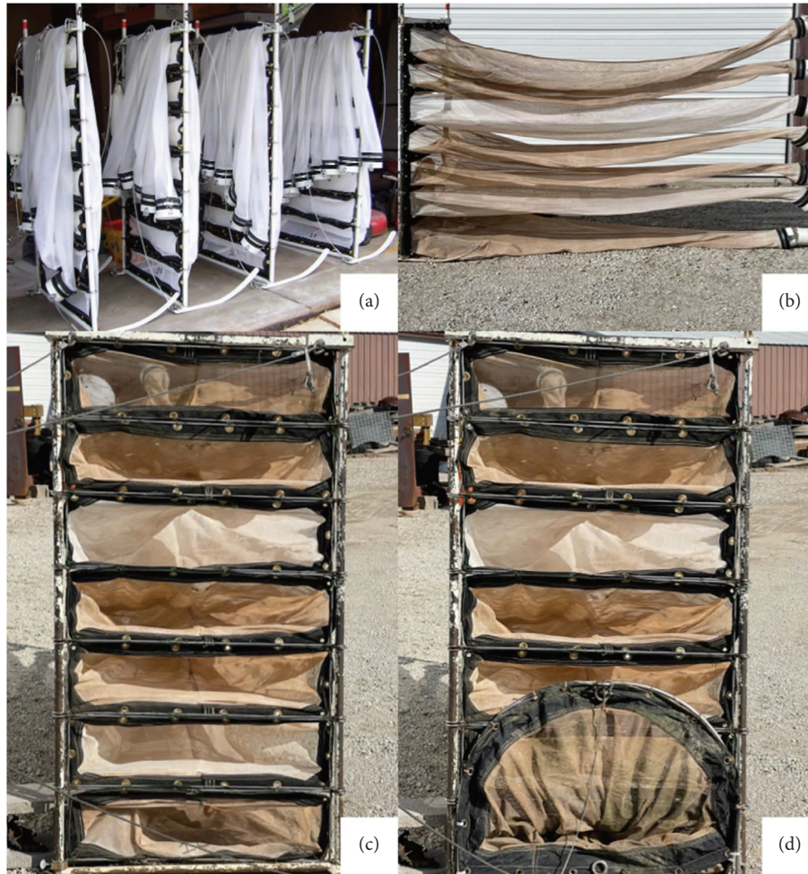
FIGURE 2: Description of the vertical nets used to sample drifting larval lake sturgeon. Panel (a) shows the 4 nets shortly after construction with backwards facing skirts and bridles, (b) provides a side view of a single vertical net with each of the 7 collection bags consisting of knotless 1.6 mm-mesh nylon (317.5 cm in length), (c) is a front view of the a vertical net which is 150 cm tall \times 76 cm wide and partitioned into 7 individual sections each 20 cm tall (net 1 is at the bottom and net 7 is at the top, and (d) provides a visual comparison vertical net against a traditional bottom sampling D-frame net.
