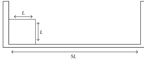
Figure 5: Schematic of the dam break problem.
