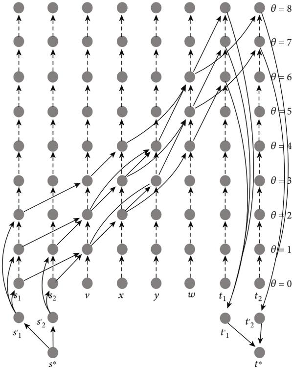
FIGURE 4: Time-expanded network of Figure 2(b).
