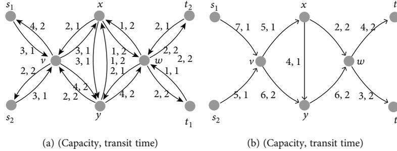
FIGURE 2: (a) Given network and (b) auxiliary network of (a).
