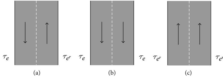
FIGURE 1: (a) represents a two-way road network, (b) represents the network, if arc  $e^r$  is reversed in the direction of arc  $e$ , and (c) represents the network, if arc  $e$  is reversed in the direction of arc  $e^r$ .
