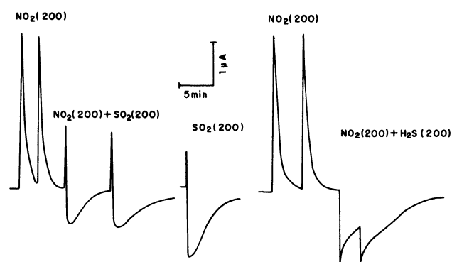
Figure 5. Effect of \text{SO}_2 and \text{H}_2\text{S} on the determination of \text{NO}_2 in FIA by the galvanic detector. The numbers represent the sample concentrations in ppm (v/v). Sample volume = 0.5 ml except for 200 ppm \text{SO}_2 : sample volume 1.0 ml.
