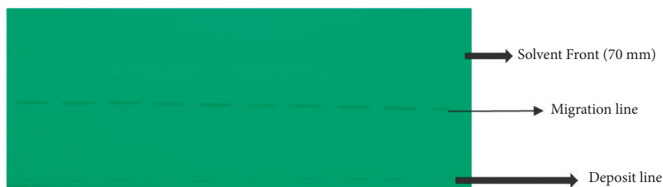
FIGURE 1: Chromatographic plate obtained with a mobile phase dichloromethane-methanol (9:1, v/v) and revealed at 254 nm.
