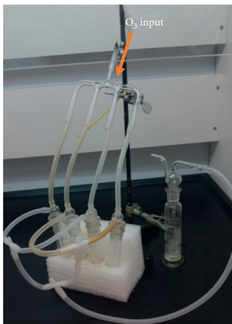
FIGURE 1: Device for the OAE. Four commercial glass (borosilicate 3.3, Pyrex ® ) midget impinger (25 mL) tubes with fritted nozzles allow to analyze a sample by triplicate and a blank simultaneously. At the bottom, a flask (trap) containing \text{Na}_2\text{S}_2\text{O}_5 solution is placed to neutralize the excess of ozone gas and close the system.
