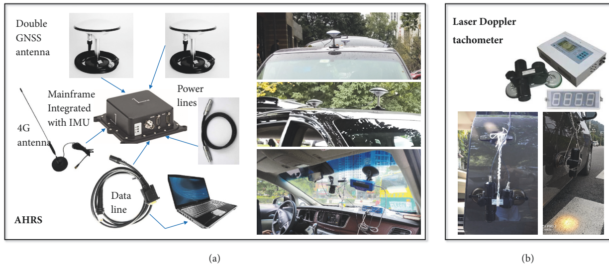
FIGURE 3: On-board equipment used in naturalistic data collection. (a) The composition of AHRS, fixed on the test car; (b) Laser Doppler Tachometer.
