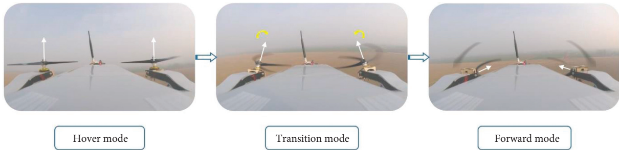
FIGURE 18: Mode transition in the flight experiment.
