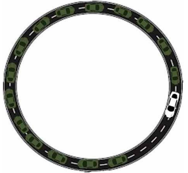
FIGURE 5: A platoon of one hundred vehicles running a circular road with length of 1500 m.
