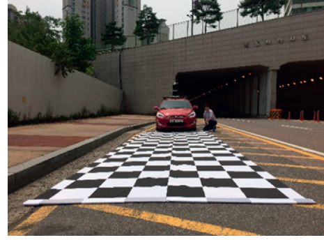
FIGURE 3: Camera extrinsic parameter calibration.
