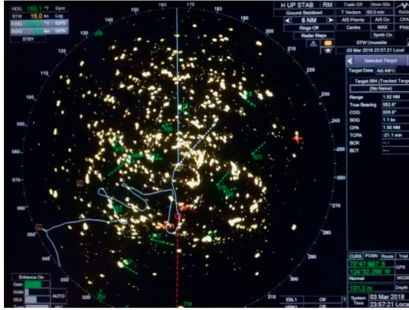
FIGURE 1: Typical radar echo image in polar ice-covered area.
