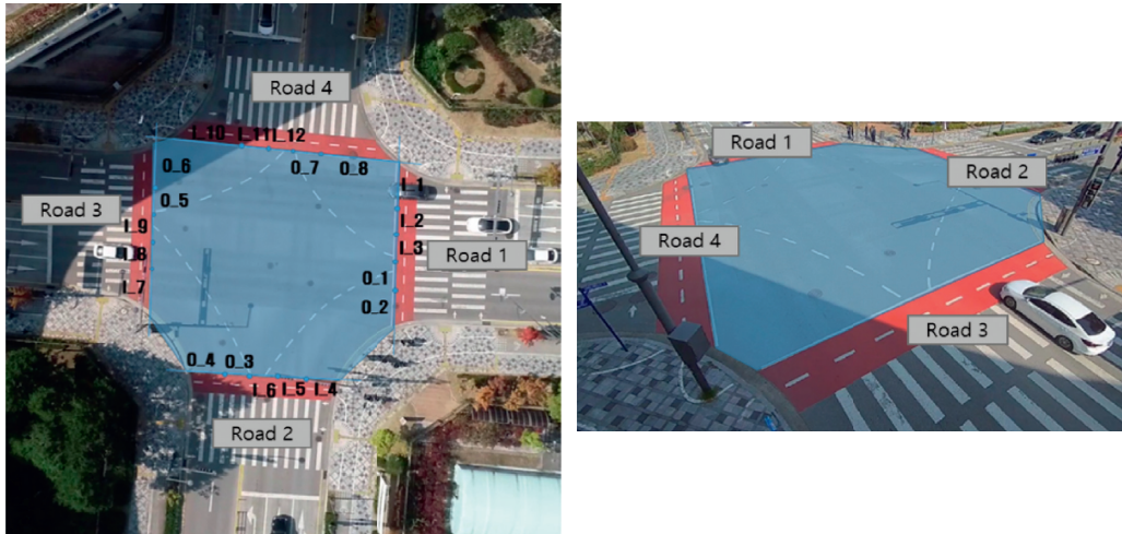
FIGURE 10: An example of comparing drone image and camera image for traffic volume estimation.
