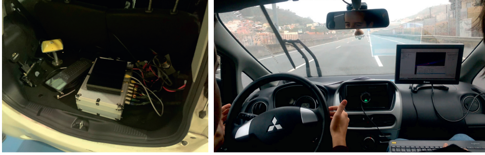
FIGURE 3: ODBII interface for controlling the vehicle and visualization of front and rear cameras for remotely controlling speed and direction.
