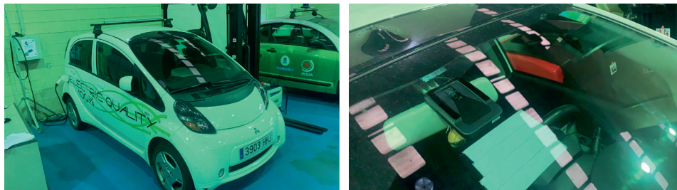
FIGURE 2: Autonomous electric vehicle used in real testing and light detection and ranging sensor (LiDAR) placed on the vehicle windscreen.
