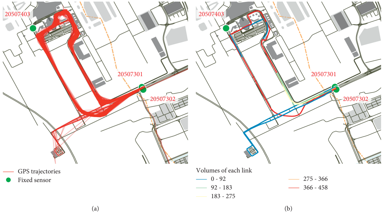
FIGURE 7: Example of realistic path generation. (a) GPS trajectories. (b) Volumes of each link.
