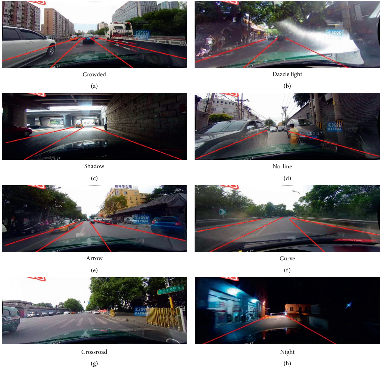
FIGURE 10: Testing on CULane. Since there is no line at crossroad, the detection result is none, as shown in (g). (a) Crowded. (b) Dazzle light. (c) Shadow. (d) No line. (e) Arrow. (f) Curve. (g) Crossroad. (h) Night.
