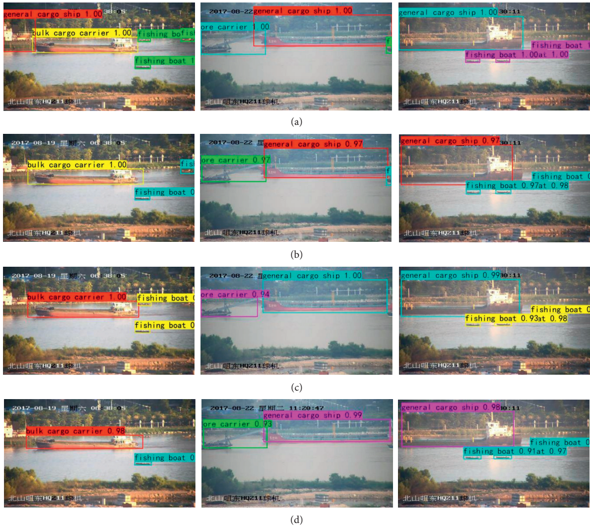
FIGURE 7: The detection results of four different algorithms on SeaShips test set: (a) AE-YOLOv3; (b) YOLOv3; (c) SSD; (d) Faster R-CNN.
