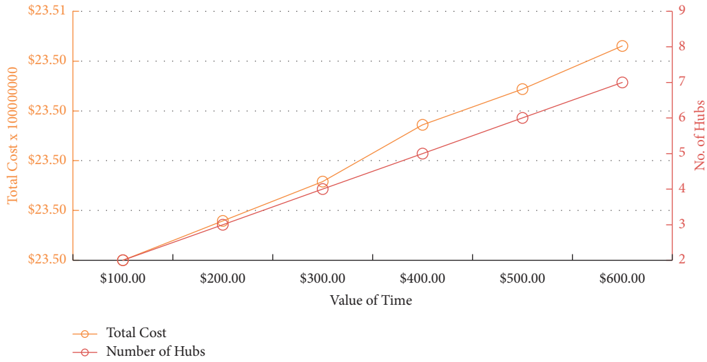
FIGURE 6: Impact of consolidation on total cost, value of time, and no. of hubs.
