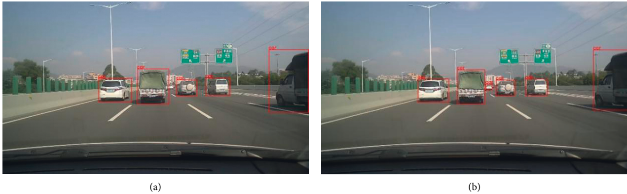
FIGURE 7: The detection results of the vehicle data set before and after the network improvement. (a) Original network target detection result. (b) Improved network target detection result.
