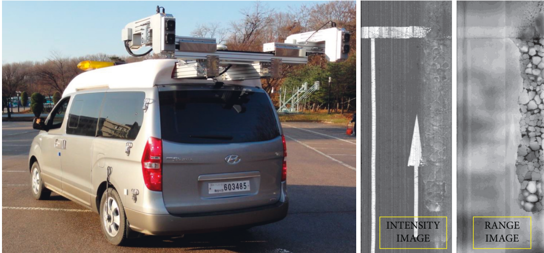
FIGURE 1: 3D laser imaging system developed by Korea Institute of Civil Engineering and Building Technology (KICT); sample of high-resolution intensity and range road surface images.
