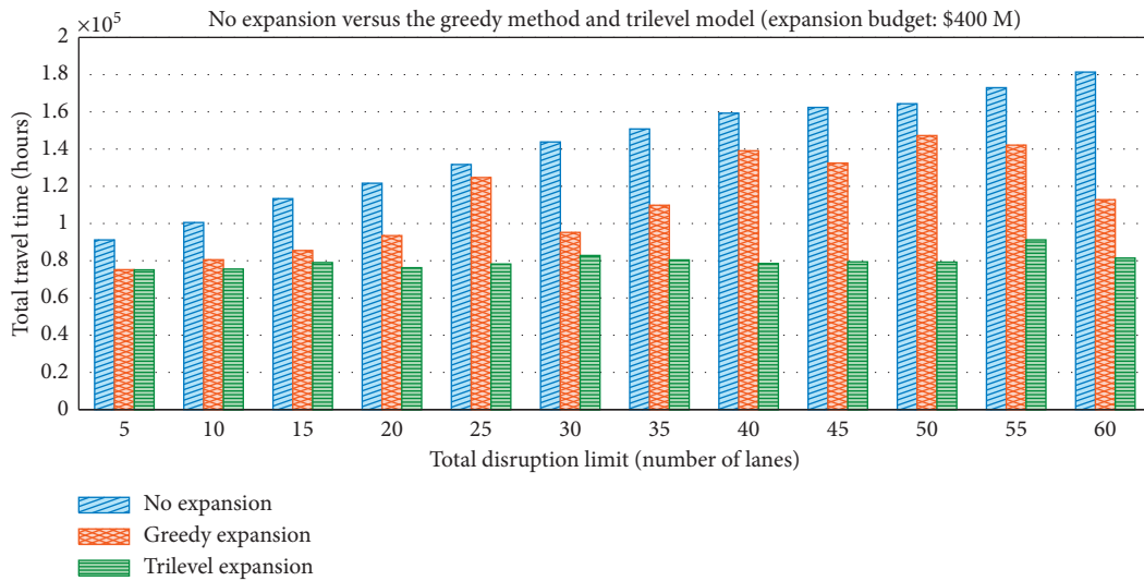
FIGURE 6: The comparison of total travel times obtained from greedy expansion and the trilevel optimization model against travel times when there is no expansion for different values of disruption limit from 5 to 60 lanes.
