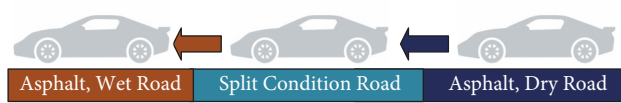
FIGURE 8: Scene of direct braking friction control under \mu -split condition of different road surfaces.
