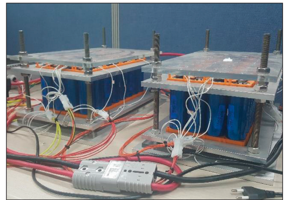
FIGURE 12: Lithium iron phosphate (LiFePO4) battery pack.
