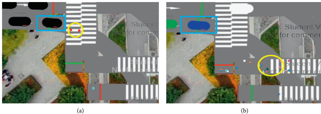
FIGURE 2: Collision between vehicles and pedestrians, the blue box represents a vehicle, the yellow box represents pedestrians. (a) The collision between a right-turning vehicle and a westbound pedestrian. (b) The collision between a right-turning vehicle and a southbound pedestrian.
