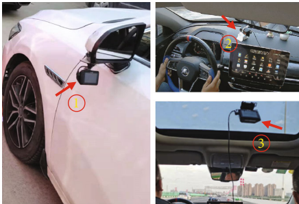
FIGURE 2: Installation location of three video cameras.
