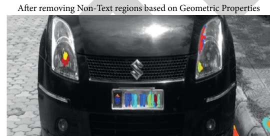
FIGURE 13: MSER blobs filtered using the geometric property.
