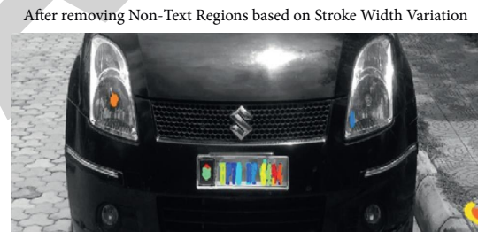
FIGURE 14: MSER blobs filtered using stroke width variation as a parameter.
