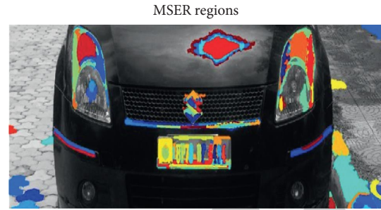
FIGURE 12: Detected MSER within a maximum and minimum threshold area.
