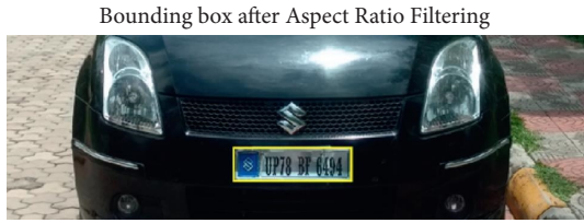
FIGURE 16: Detected number plate after aspect ratio filtering.
