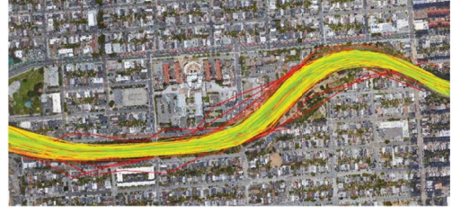
FIGURE 4: Visualization of the standard deviation of the distance between trajectory points and the road centerline.
