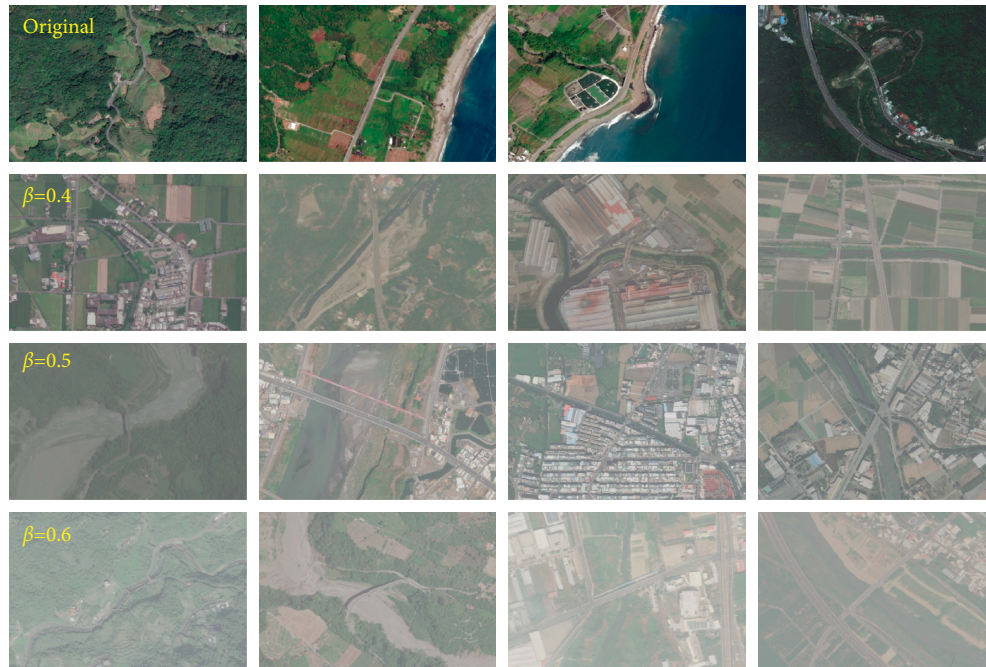
FIGURE 5: The displays of original images and their hazy versions. From top to bottom: original sharp images and hazy images with \beta = 0.3 , \beta = 0.4 , and \beta = 0.5 , respectively. In particular, \beta denotes the scattering coefficient. In addition, the global airlight A is set to 0.7 in these images.
